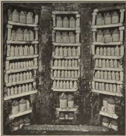
FIG. 119. — The interior of a pottery kiln.
